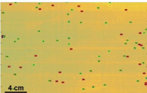
Detected defects in the coating process, red: high  $T^2$  values, green: high residual values
