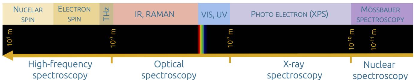
*Overview of the electromagnetic spectral range and the associated spectroscopic methods*
